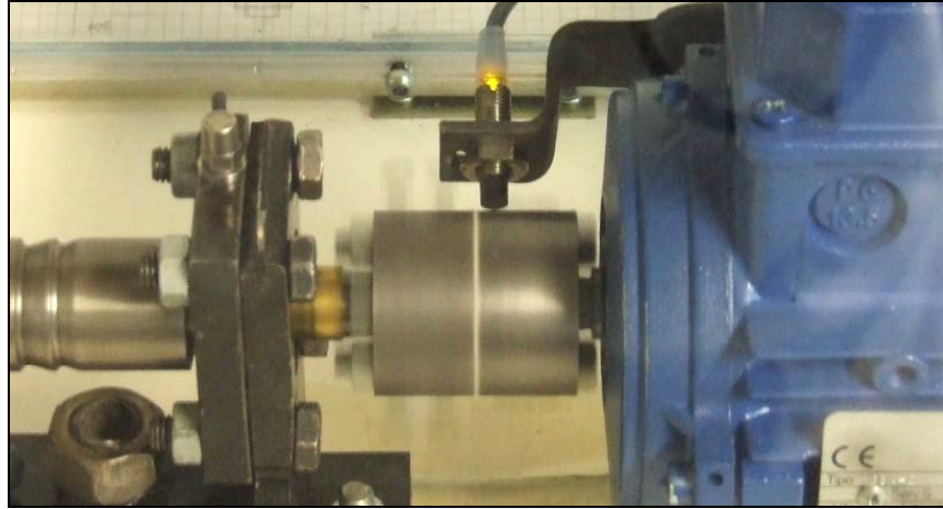
FIGURE 7. Coupling and inductive sensor
