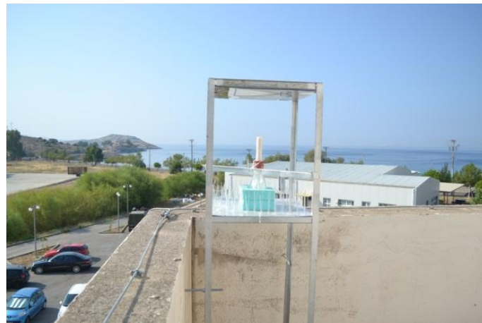
FIGURE 2. Device used for “Determining Atmospheric Chloride Deposition Rate by Wet Candle Method” at the airport. Facing the sea in a distance of 150 m from the seacoast
