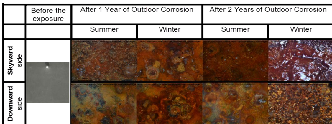
FIGURE 9. Corrosion products developments on steel surface observed by OM.
