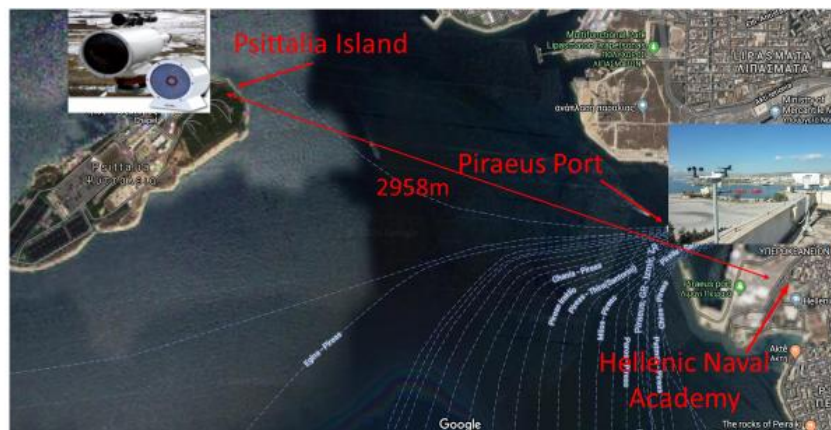
FIGURE 7. The maritime optical communications link that connects the Hellenic Naval Academy and the lighthouse on Psitalia Island and has a total length of 2958 meters [10].
